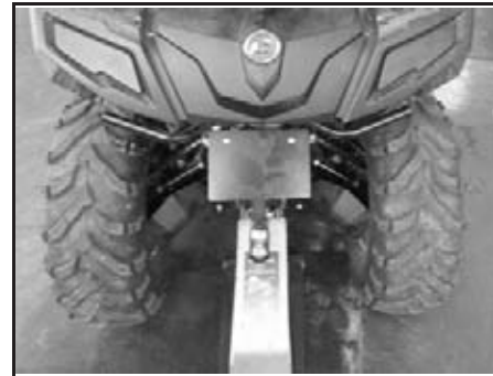
TYPICAL BACK UP POINT LOCATION
