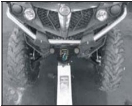
TYPICAL FRONT UP POINT LOCATION
