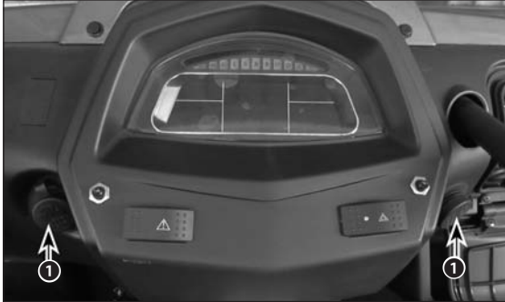
1. 12V DC outlets
